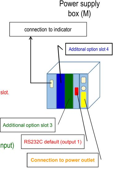
Additional option slot 4: Relay contact (FS-LM) can be installed here.
