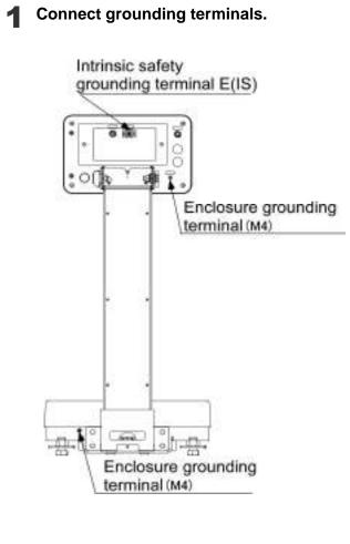
In this product the internal circuit is electrically connected with the enclosure.
