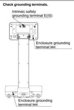
Make sure that there is no looseness, rust or damages on the ground terminals.
