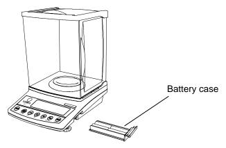
The Image icon is displayed when the balance is operated on batteries. As the batteries get weaker, the icon changes to • (flashing). When the icon changes to • (flashing), recharge or replace the batteries.
