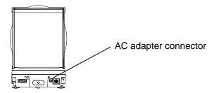
After the balance has been moved, open the windshield door to allow it to adapt to the ambient temperature for stable measurement. In addition, allow five minutes after turning on the power for the balance to warm up.
