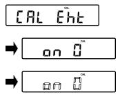
The indication changes to the flashing of "CAL EHT", "on 0", and then "on 0", followed by the starting of the zero-point adjustment.
