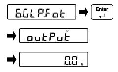
Push the [Direction] key. Select "6.GLP.FOT". Push the [Enter] key.
